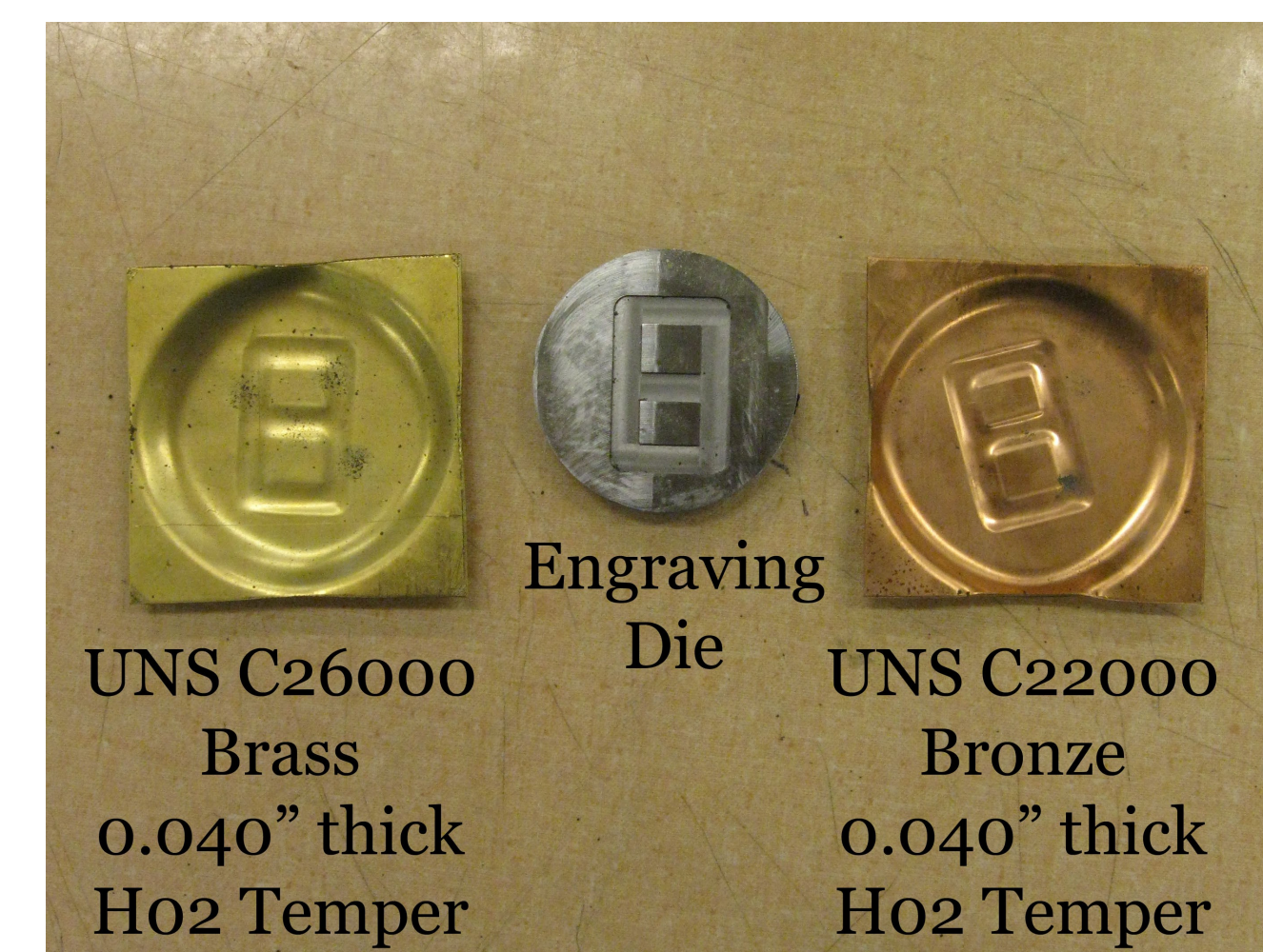
Figure 3: Explosively Formed Blanks and Engraving Die
